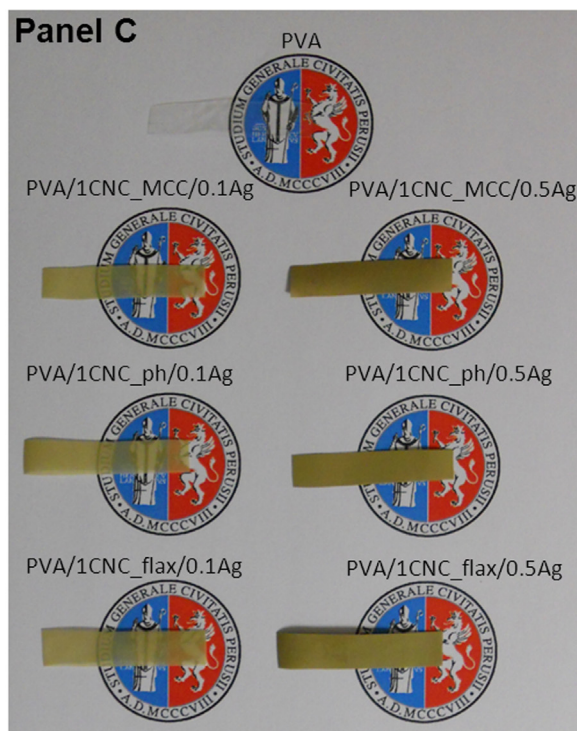
Fig. 3. UV–vis analysis (panel A), transmittance values at 700 nm (panel B) and visual observation of the solvent casting of PVA and PVA ternary bio-nanocomposites.
